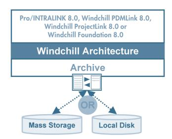
Windchill Archive works with all Windchill-based solutions (including Pro/INTRALINK 8.0) providing a means to extract and restore product information.
